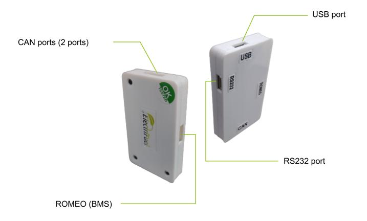
**USB port**: The USB port in OBD connects diagnostic tools or computers to the BMS system, enabling data transfer between the OBD system and external devices.
